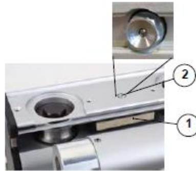
Fig. 22 Lubrication point for the Guide shaft lubrication, (1): felt strip, (2): grease nipple
