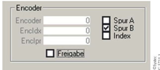
Fig. 20 Encoder group box when activated; enable [= Freigabe] not yet activated.
