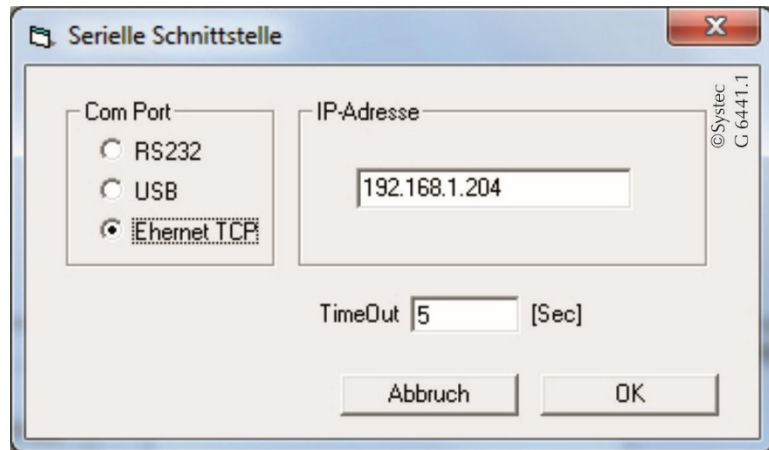
Abb. 2 Configuration of the interface, in the example of the Ethernet interface by entering the IP address and the timeouts.
