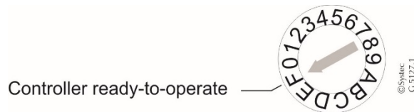
Fig. 23 Operation switch on the Xemo controller at position "F".
