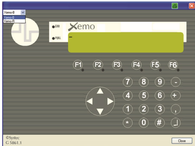
Fig. 57 Virtual display for testing the programming; in the upper left corner, you can choose between the display for Xemo R and Xemo B.
