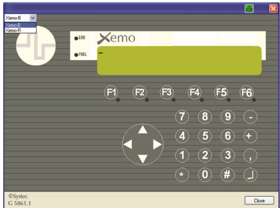
Fig. 25 Simulation of the Xemo controller's interface
